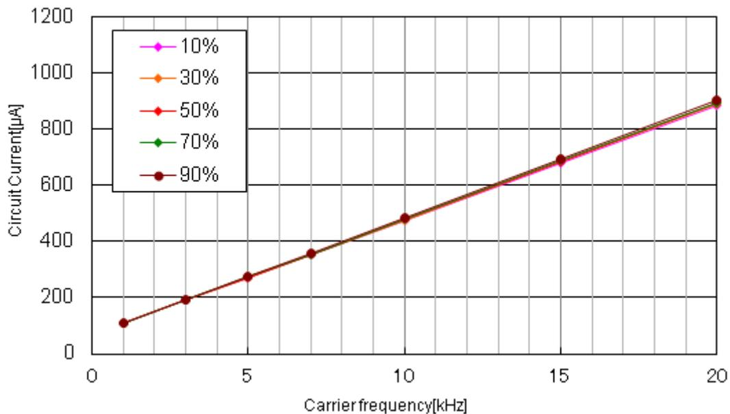
Figure 4.4.3 BM64377S (600V/30A) IBS- Carrier Frequency  $f_c$
