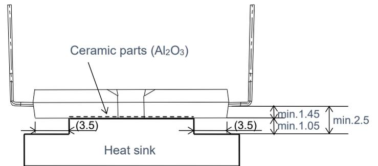
Figure 2.1.2 In the case of using the convex heat sink (unit: mm)
