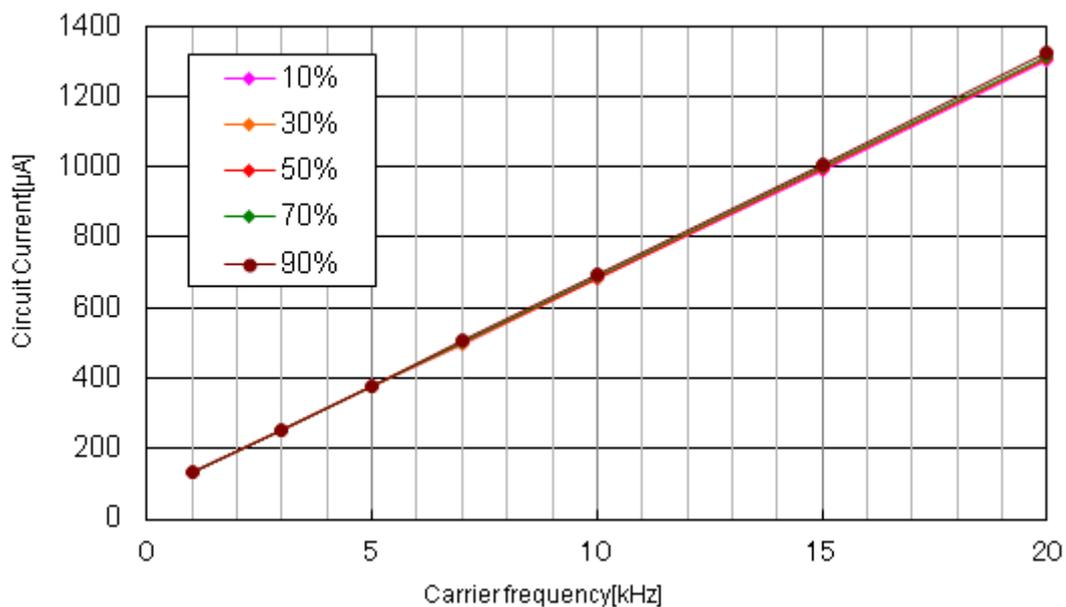
Figure 4.4.4 BM64378S (600V/35A) IBS- Carrier Frequency  $f_c$
