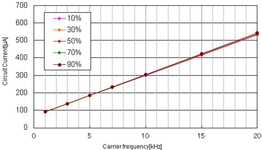
Figure 4.4.1 BM64374S (600V/15A)  $I_{BS}$ - Carrier Frequency  $f_c$
