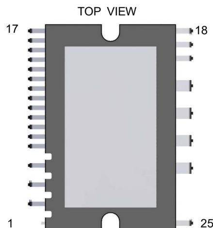
Figure 2.3.2 Pin Configuration
