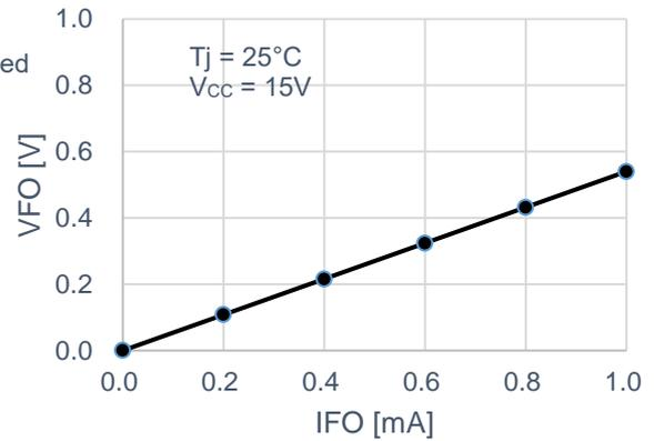
Figure 2.2.13 FO pin V-I characteristics
