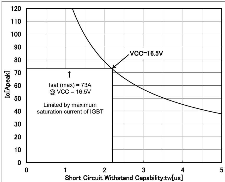
Figure 3.8.2 Typical BM64374S (15A) SCSOA curve
