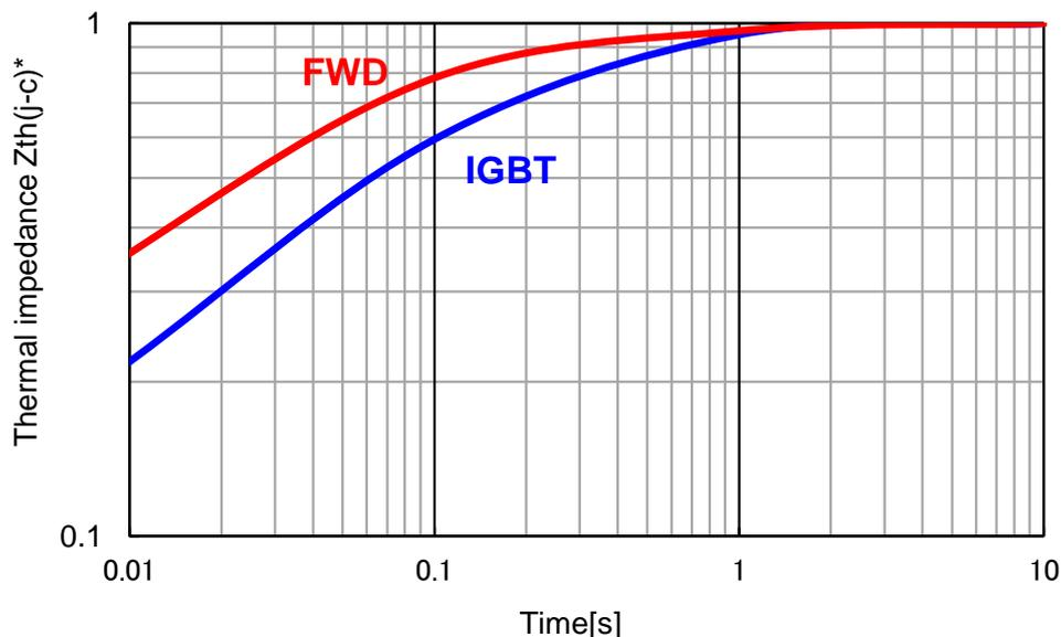
Figure 2.1.3. Transient Thermal Impedance
