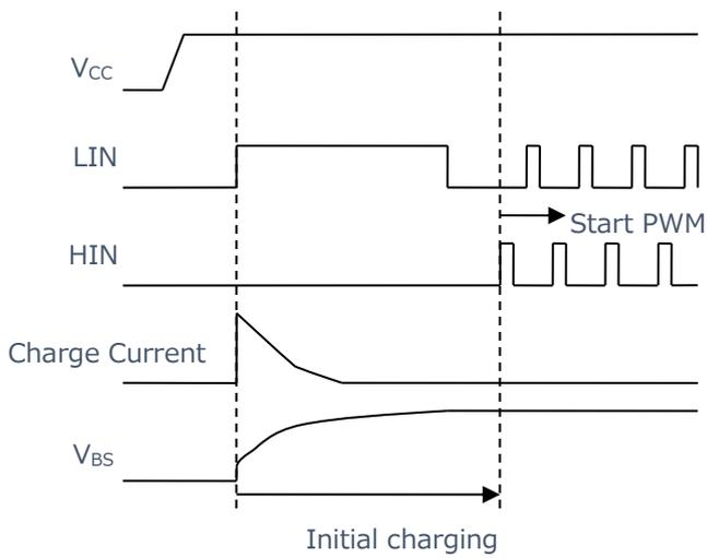
Figure 4.2.1 Waveform by one charging pulse
