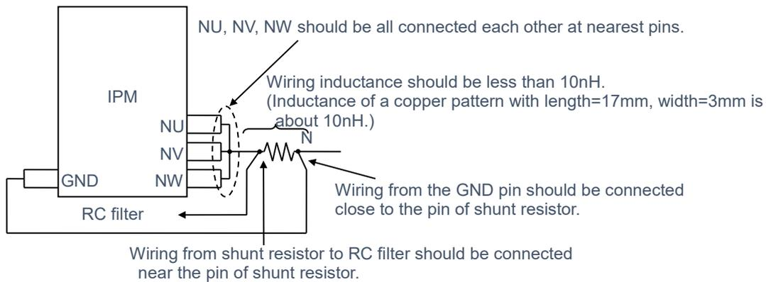
Low inductance shunt resistor like surface mounted (SMD) type is recommended.
