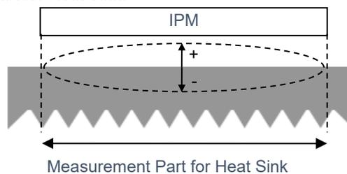
Figure 2.3.7 Measurement Point of Heat Sink Flatness
