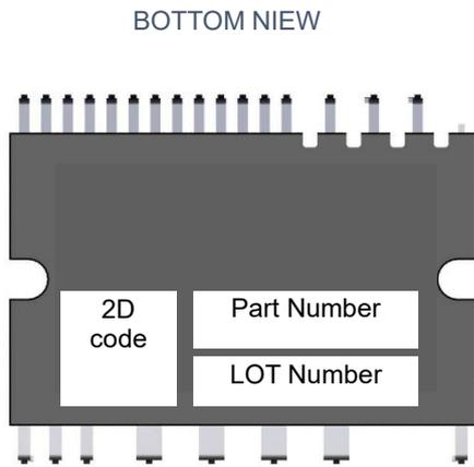
Figure 2.3.3 Marking Diagram
