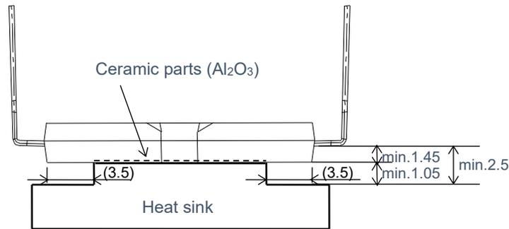
Figure 2.3.4 In the case of using the convex heat sink (unit: mm)
