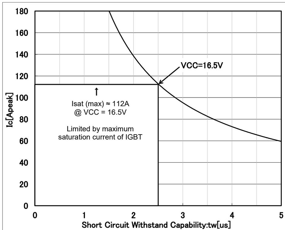
Figure 3.8.3 Typical BM64375S (20A) SCSOA curve
