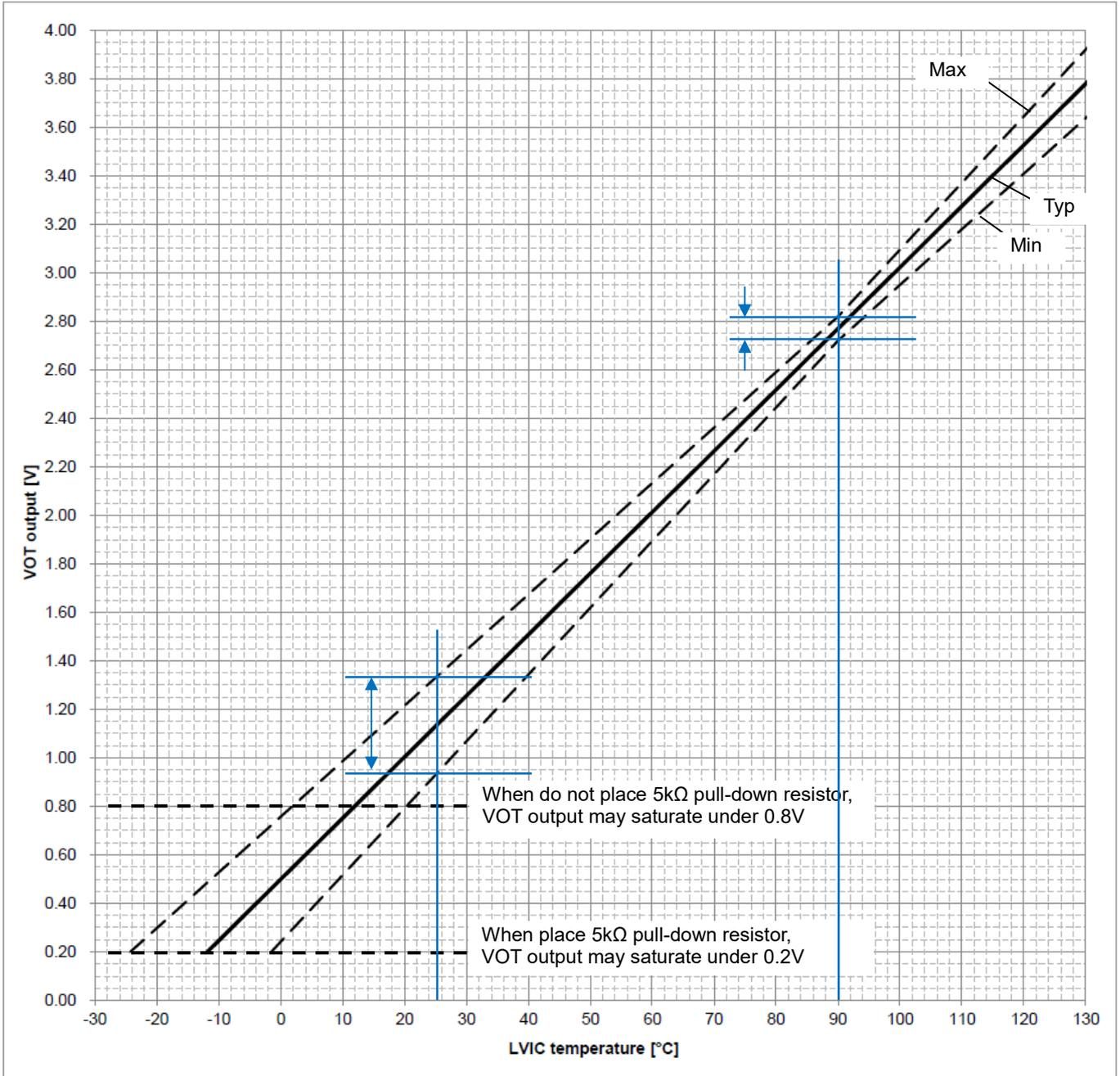
Figure 2.2.11 VOT Output vs LVIC temperature Characteristics
