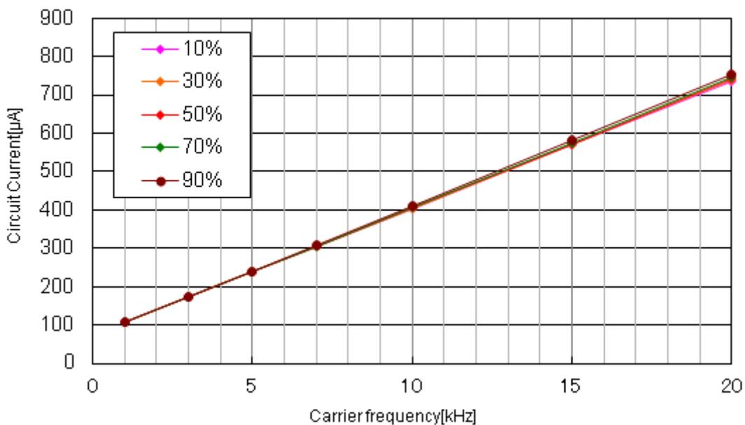
Figure 4.4.2 BM64375S (600V/20A)  $I_{BS}$ - Carrier Frequency  $f_c$
