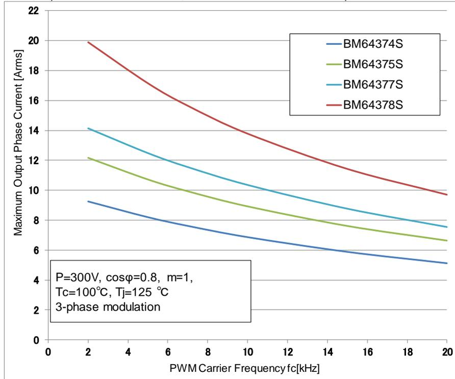
Figure 3.7.1  $I_o$ -carrier frequency characteristics
