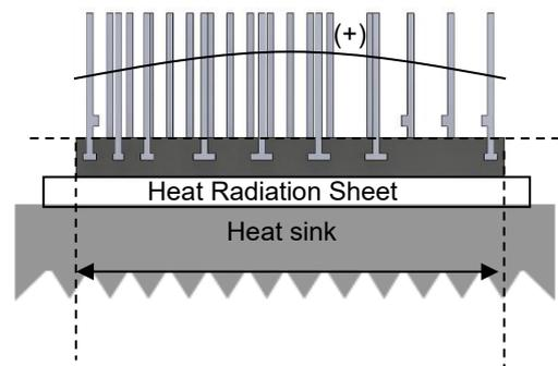
Figure 2.3.5 Flatness after Installing to a Heat sink (When Using a Heat Radiation Sheet)
