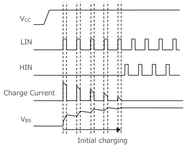
Figure 4.2.2 Waveform by multiple charging pulses
