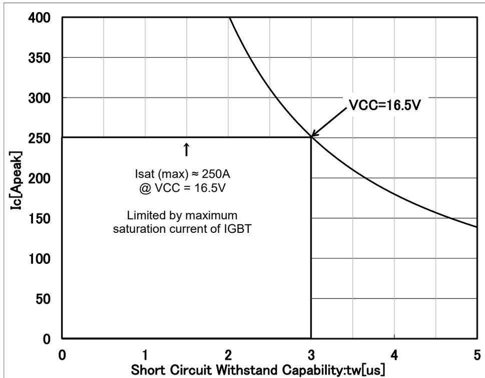
Figure 3.8.5 Typical BM64378S (35A) SCSOA curve
