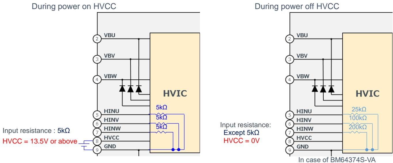
Figure 2.2.17 Input resistance equivalent block diagram
