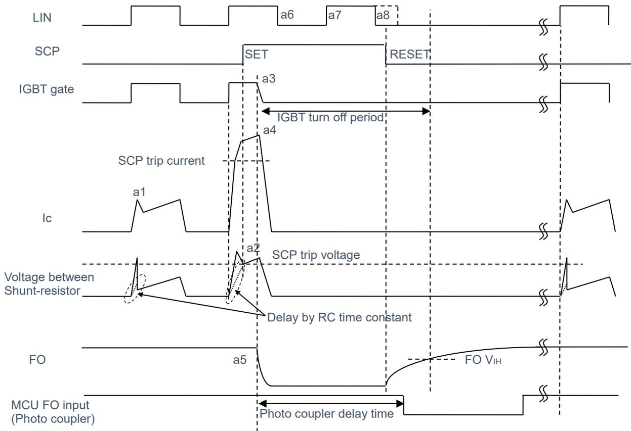
Figure 2.2.16 Extension IGBT turn off period timing chart
