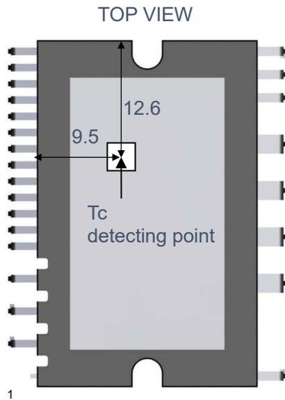
Figure 2.1.1 Tc Detecting Point (unit: mm)
