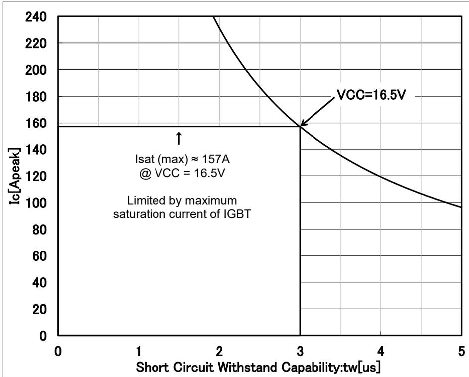
Figure 3.8.4 Typical BM64377S (30A) SCSOA curve
