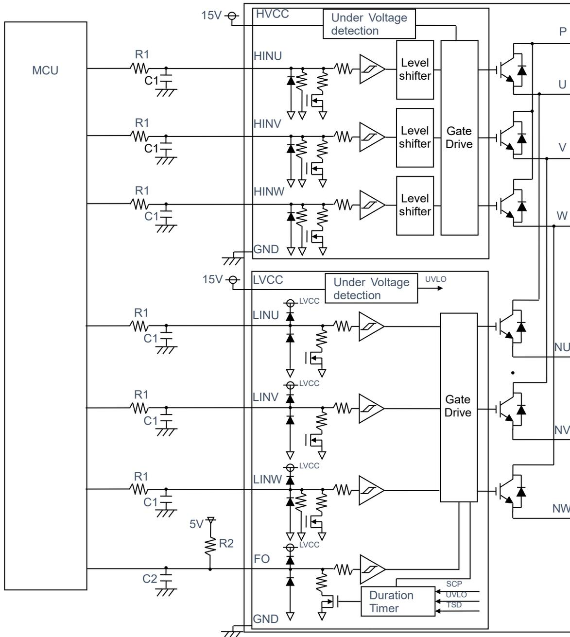
Figure 2.2.12 FO pin and other control pins
