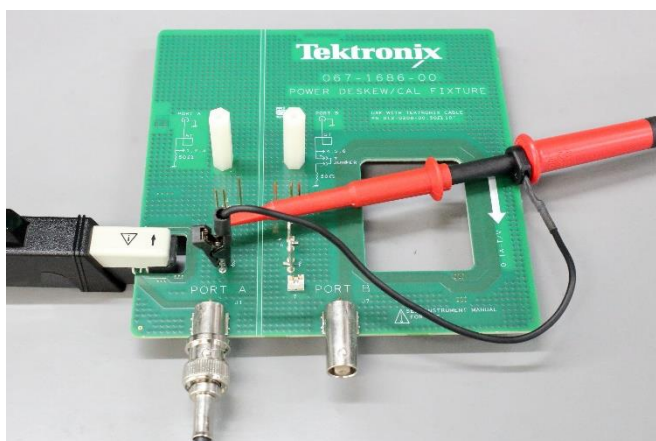
Figure 5. Deskew fixture made by Tektronix
