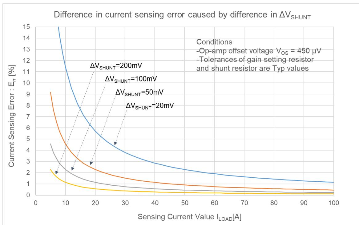
Figure 6. Effect of difference in  $\Delta V_{SHUNT}$  on the current sensing error
