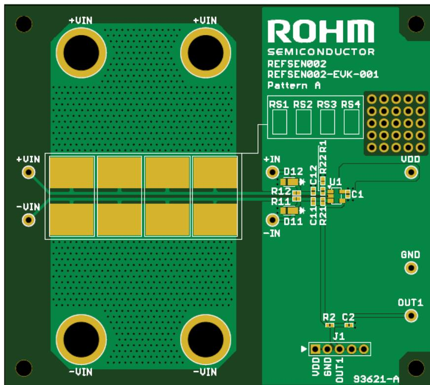
Figure 5. PCB Layout of Reference Design [REFSENS002]
