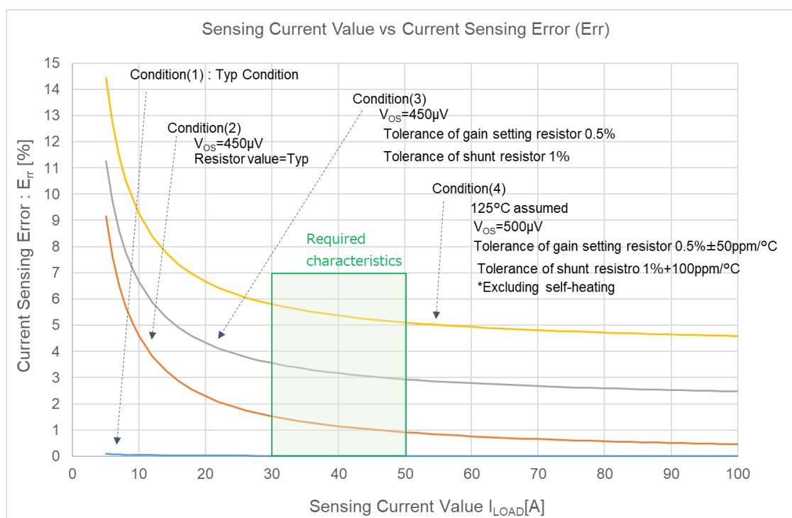
Figure 3. Current sensing error vs. sensing current value for the designed circuit
