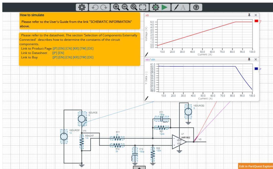
Figure 4. Simulation circuit example on ROHM Solution Simulator
