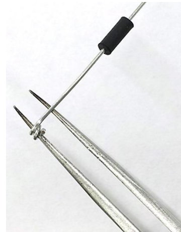
Figure 9. Creating the tip (end) support part of the adapter
