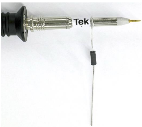
Figure 8. Creating the ground support part of the adapter
