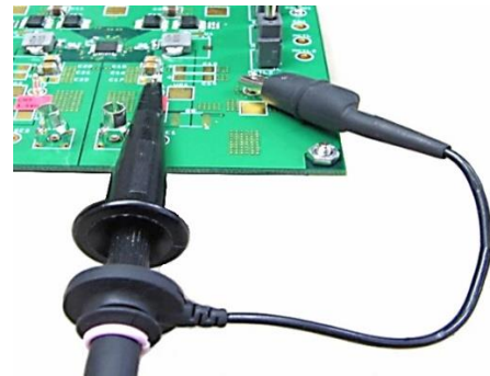
Figure 1. Monitoring of switching location with voltage probe; the ground side connected with the ground lead with attached alligator clip.
