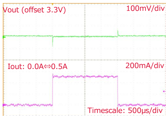
Figure 34 Load response of LDO_P5V_S3V3
