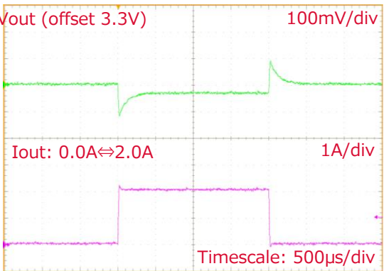
Figure 31 Load response of DCDC_P3V
