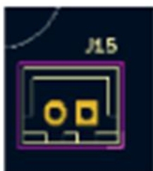
Figure 3-2. Built-in thermistor connector (top view)
