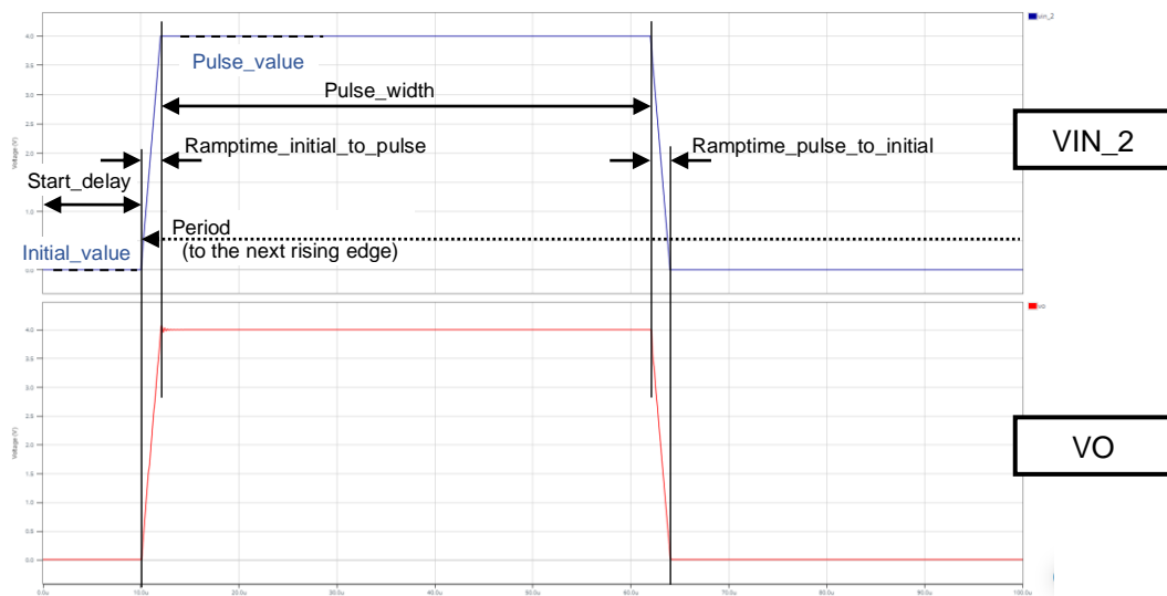
Figure 3. VSOURCE parameters and its waveform
