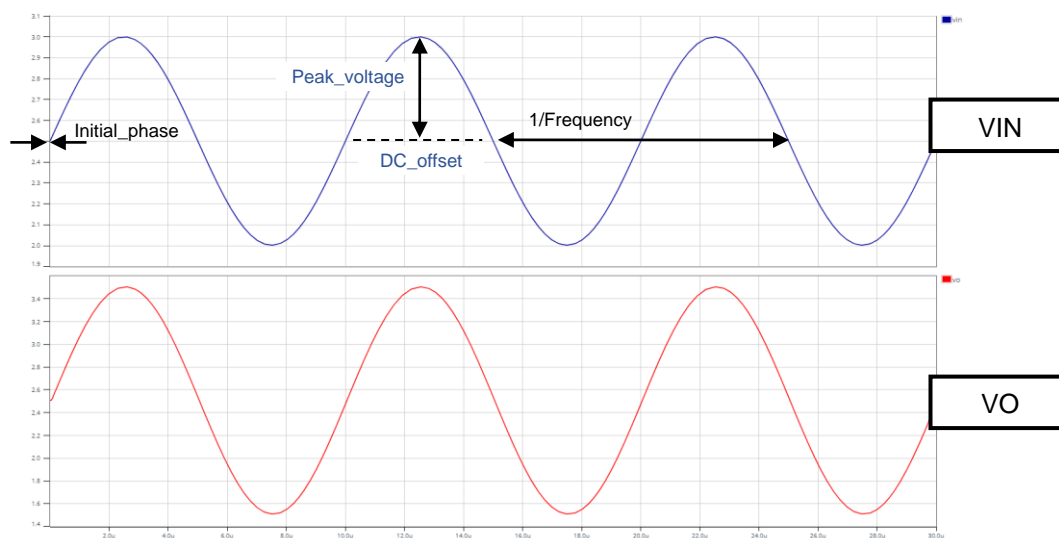
Figure 3. VSOURCE parameters and its waveform
