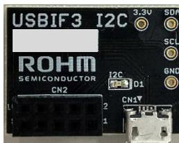
Note: USB cable(USB-A to Micro-B) is required due to connect PC.
