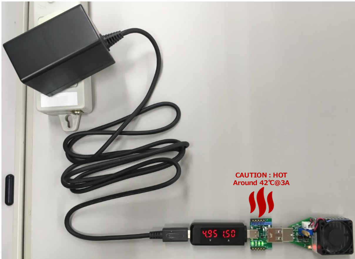
<An example of the actual evaluation with USB C adapter, Type-C Meter, the EVK, and USB load>
