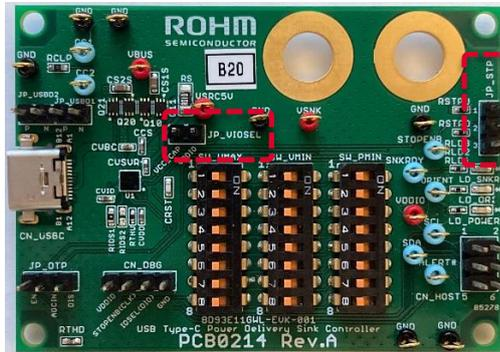
2. Short EN and ADCIN on JP\_TOP if the Over Temperature Protection with the external PTC thermistor is in use. If not in use, short ADCIN and SGND.
