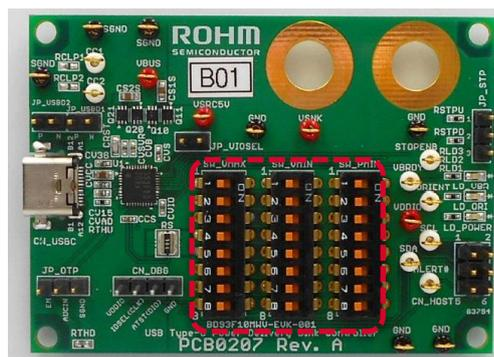
4. When connecting the existing system board for evaluation, connect the EVK into the existing system board before power up as shown in Figure 6.
