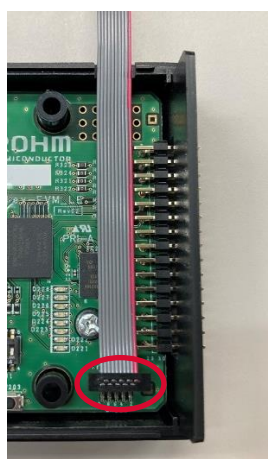
Figure 4. Debug I/F Terminal and cable direction
