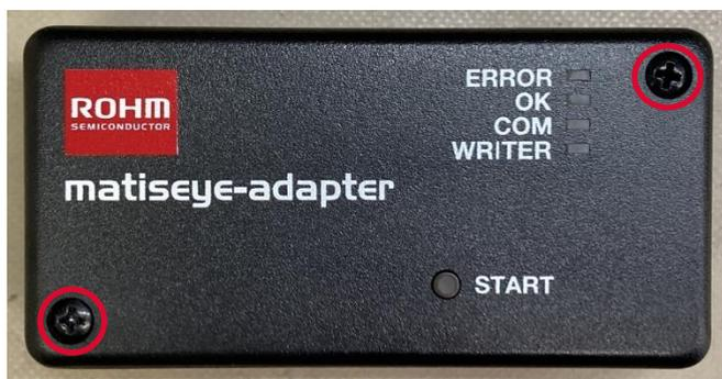
Figure 4. Positions of Screws
