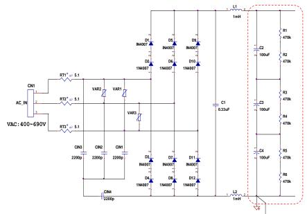
Figure 1-5. Input capacitor and Balance resistance
