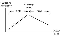
Figure 1-1.Switching Frequency – Output Load Characteristics
