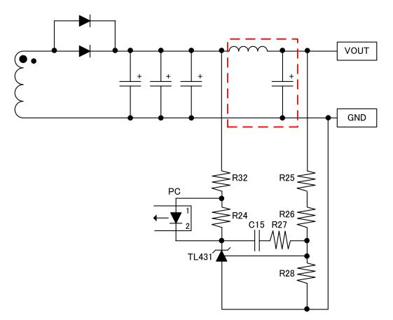
Figure1-11. LC Filter Circuit
