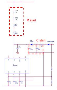
Figure1-9. resistance of Starter and VCC capacitor
