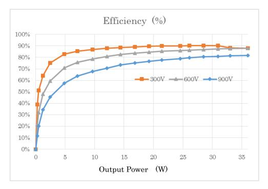
Figure 2-2. Efficiency vs Output Power
