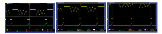
VIN(DC)=300V VIN(DC)=600V VIN(DC)=900V Figure 2-4. Drain Voltage and Drain current waveform (VO=24V,IO=1.0A, PO=24W) CH1: Vdrain (200V/div), CH4: Idrain (200mA/div)
