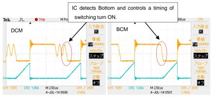
Figure 1-2.Switching waveform (MOSFET Vds,Ids)
