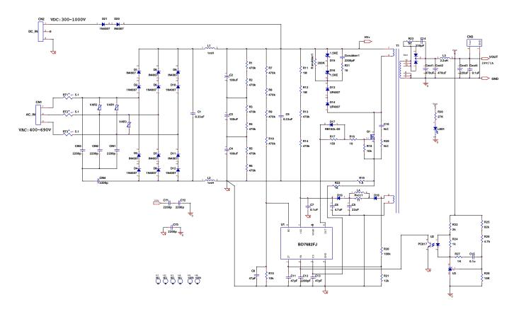
Figure 2-1. Isolated Fly-buck Quasi-Resonant convertor(24V1A=24W)
