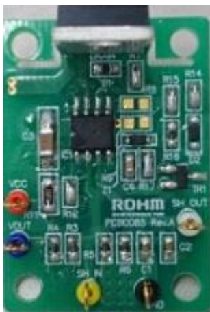
Figure 1. BM1R00147F-EVK-001 Evaluation Board
