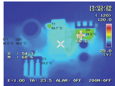
Figure 50. Thermal Image VIN:264 Vac, IOUT:4 A
