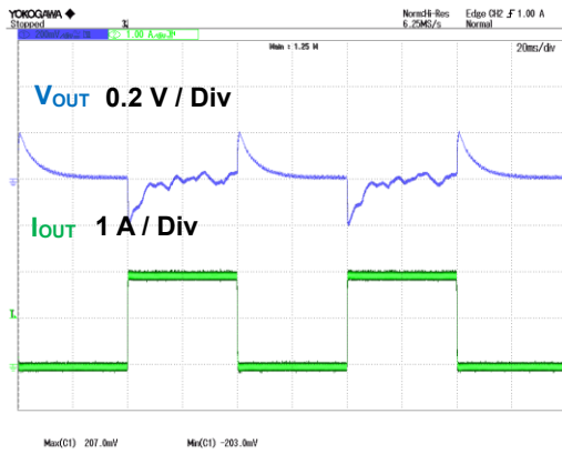
Figure 19. V_{IN} = 90 \text{ Vac} , I_{OUT} = \text{switch } 0.06 \text{ A} / 2 \text{ A}
