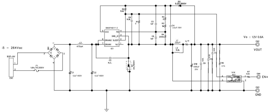
Figure 4. Application Circuit
