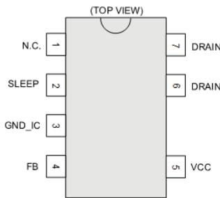
Figure 7. Pin Configuration
