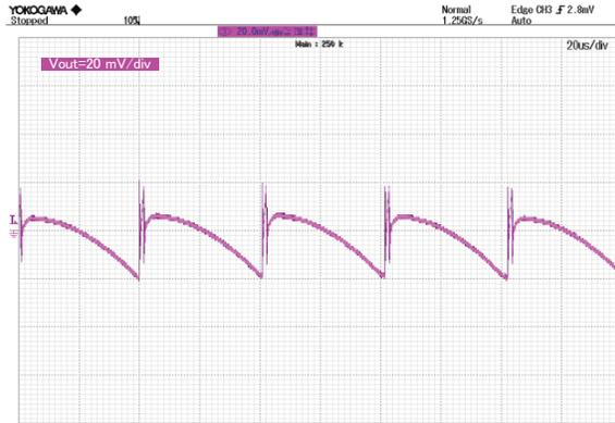
Figure 26. Vout Ripple Voltage (5MHz filter)
