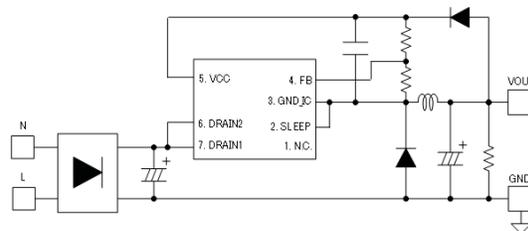
Figure 2. BM2PAB1Y-EVK-001 Simple Schematic
