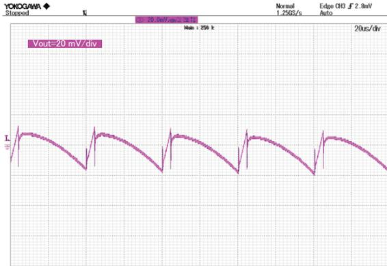
Figure 25. Vout Ripple Voltage (5 MHz Filter)
