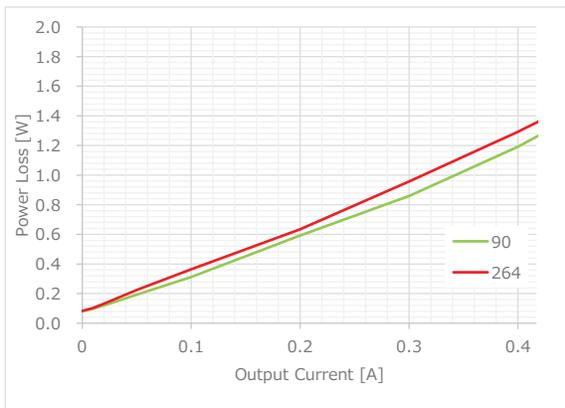
Figure 10. IOUT vs. Power Loss
