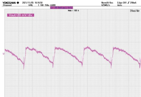
Figure 26. Vout Ripple Voltage (5MHz filter)
