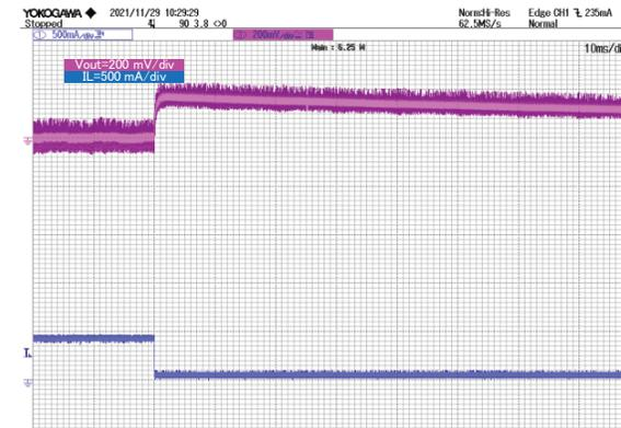
Figure 24. Iout and Vout (5 MHz Filter)
