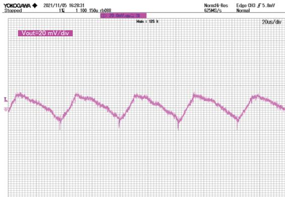
Figure 25. Vout Ripple Voltage (5 MHz Filter)
