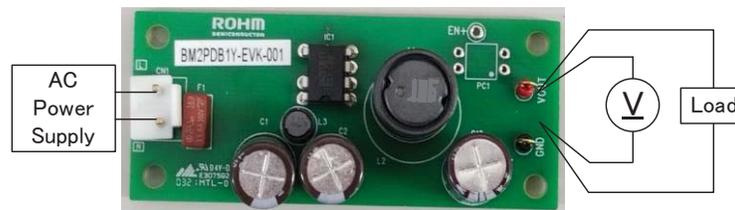
Figure 3. Connection Circuit
