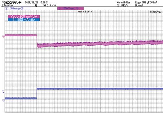
Figure 21. Iout and Vout (5 MHz Filter)
