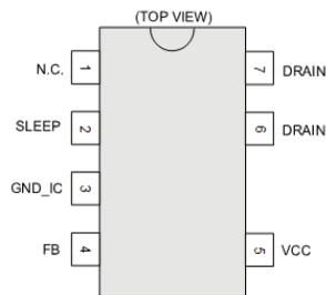
Figure 7. Pin Configuration
