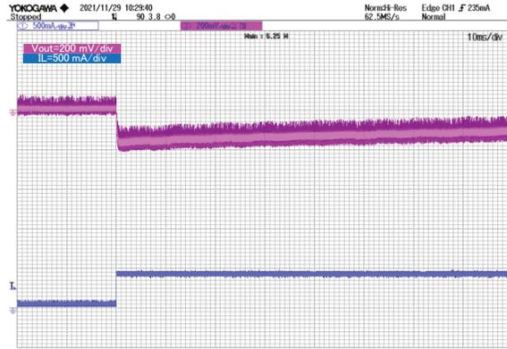
Figure 22. Iout and Vout (5 MHz Filter)
