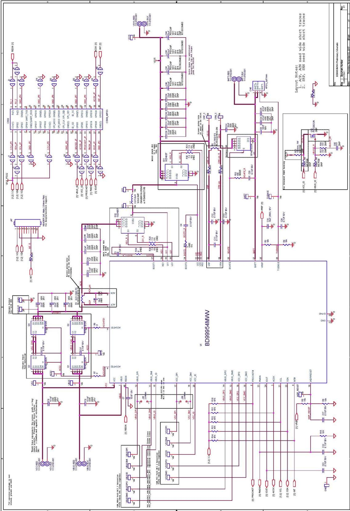
Figure 33. BD99954 Reference Schematic
