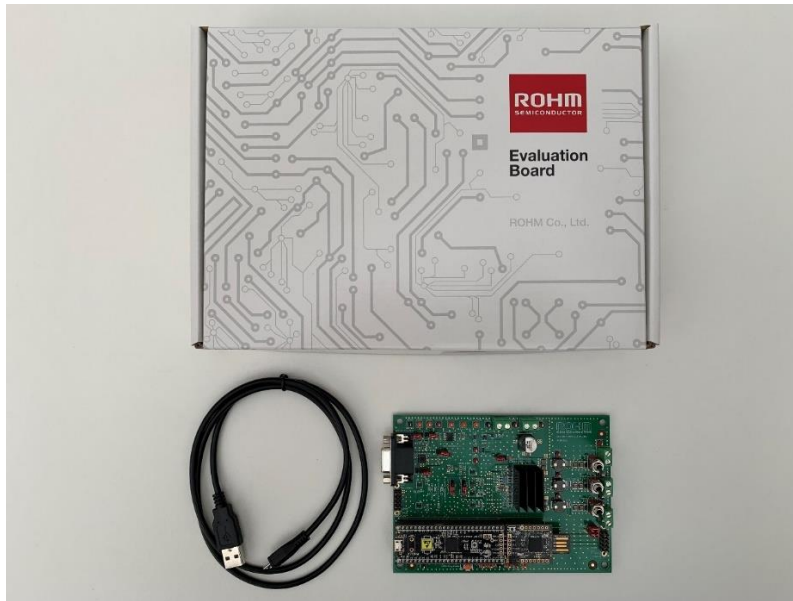
Figure 1. BD18397/98RUV-EVK-302 Evaluation Kit Contents
