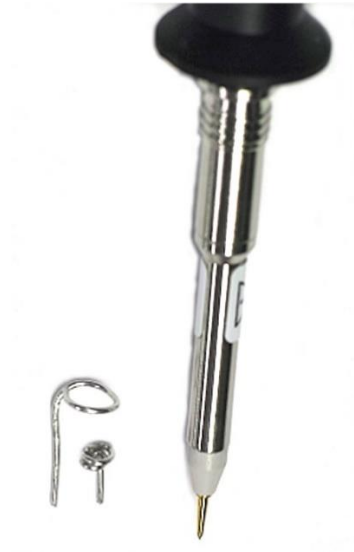
Figure 10. Created simplified probe tip adapter
