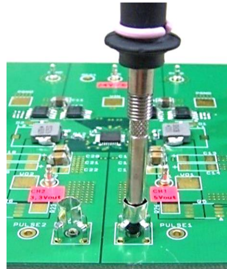
Figure 6. State where the switching location is monitored using the probe tip adapter
