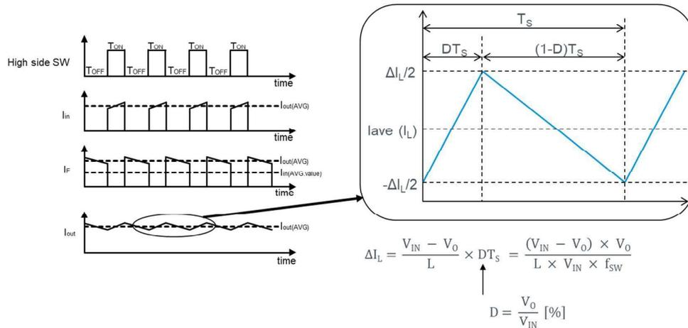
Figure 3. Illustration of Ripple Current
