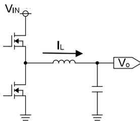
Figure 1-b. Synchronous Buck Converter
