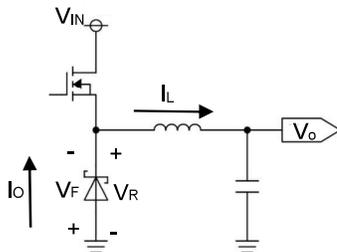
Figure 1-a. Asynchronous Buck Converter
