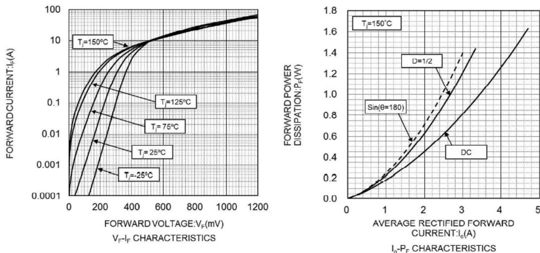
Figure 4. Rohm Schottky Barrier Diode RSX301LAW30 Characteristic Curve for Forward Loss
