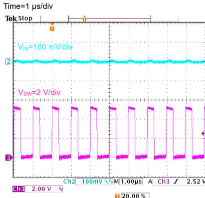
Figure 16. Input Voltage Ripple
