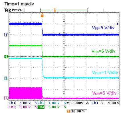
Figure 11. Shutdown at  $R_{LOAD} = 0.9 \Omega$
