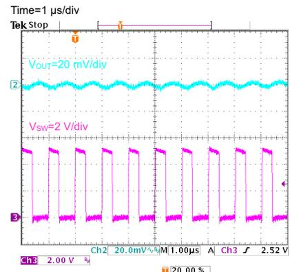
Figure 15. Output Voltage Ripple
