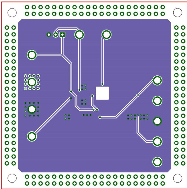
Figure 9. Bottom Layer Layout (Top View)
