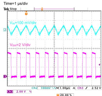
Figure 17. Input Voltage Ripple
