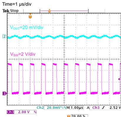
Figure 14. Output Voltage Ripple
