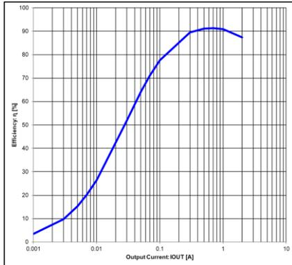
Figure 18. Efficiency vs Output Current ( $V_{IN} = 5\text{ V}$ ,  $V_{OUT} = 1.8\text{ V}$ )
