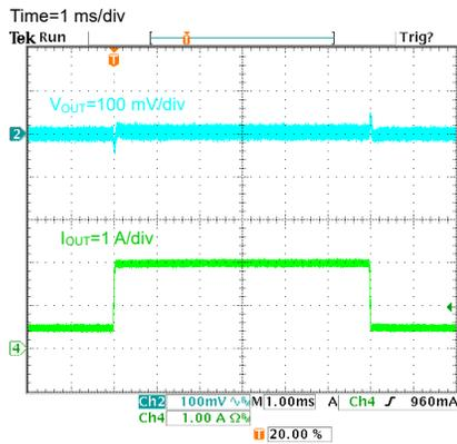
Figure 20. Load Transient Response ( $V_{IN} = 5\text{ V}$ ,  $V_{OUT} = 1.8\text{ V}$ ,  $I_{OUT} = 0.5\text{ A to }2.0\text{ A}$ )
