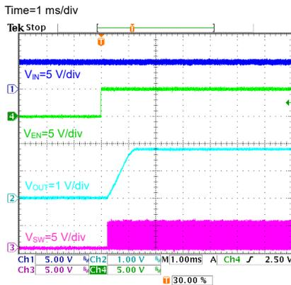
Figure 12. Start-up at  $R_{LOAD} = 0.9 \Omega$
