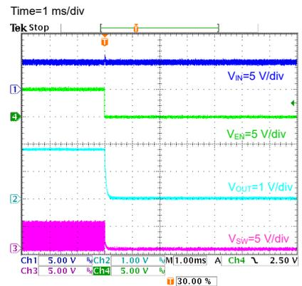
Figure 13. Shutdown at  $R_{LOAD} = 0.9 \Omega$
