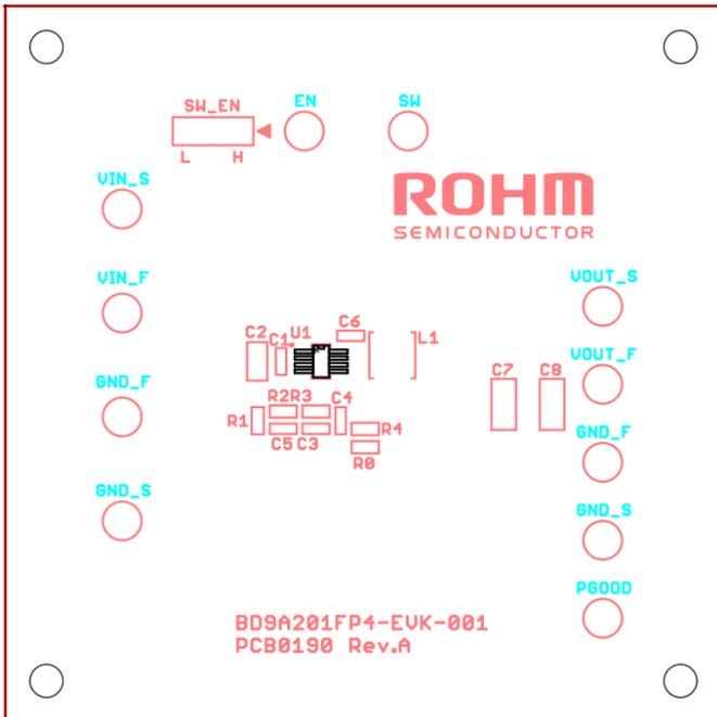
Figure 5. Top Silkscreen Layout (Top View)
