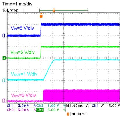
Figure 10. Start-up at  $R_{LOAD} = 0.9 \Omega$
