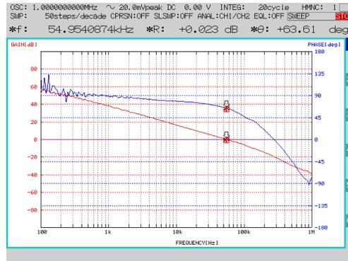
Figure 19. Frequency Characteristics ( $V_{IN} = 5\text{ V}$ ,  $V_{OUT} = 1.8\text{ V}$ ,  $I_{OUT} = 1\text{ A}$ )
