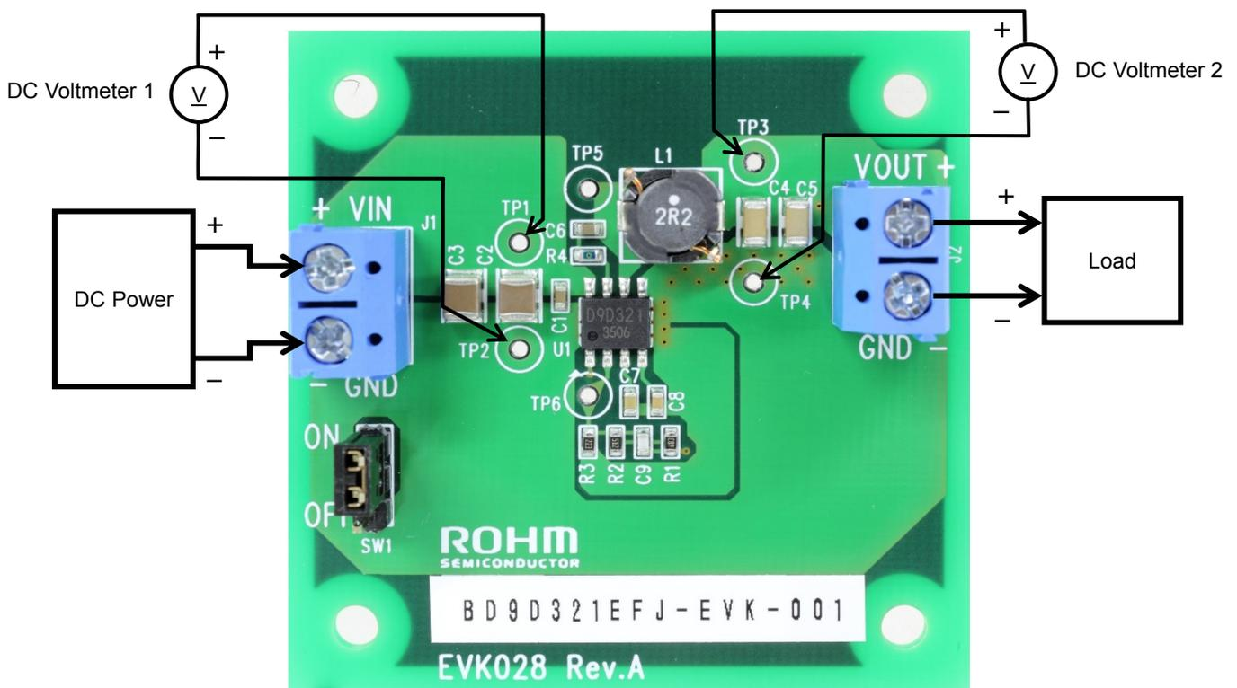
Figure 1. Connection Diagram
