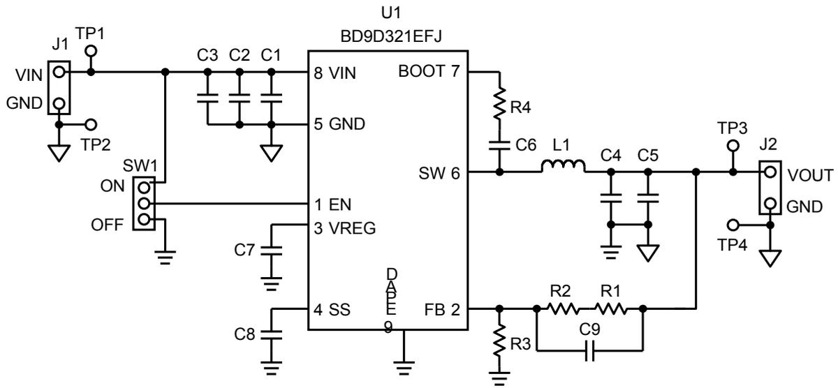
Figure 2. BD9D321EFJ-EVK-001 Circuit Diagram
