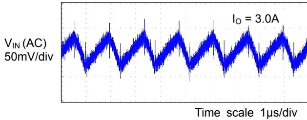
Figure 13. Input Voltage Ripple Wave
