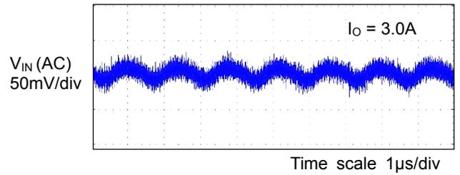
Figure 14. Output Voltage Ripple Wave
