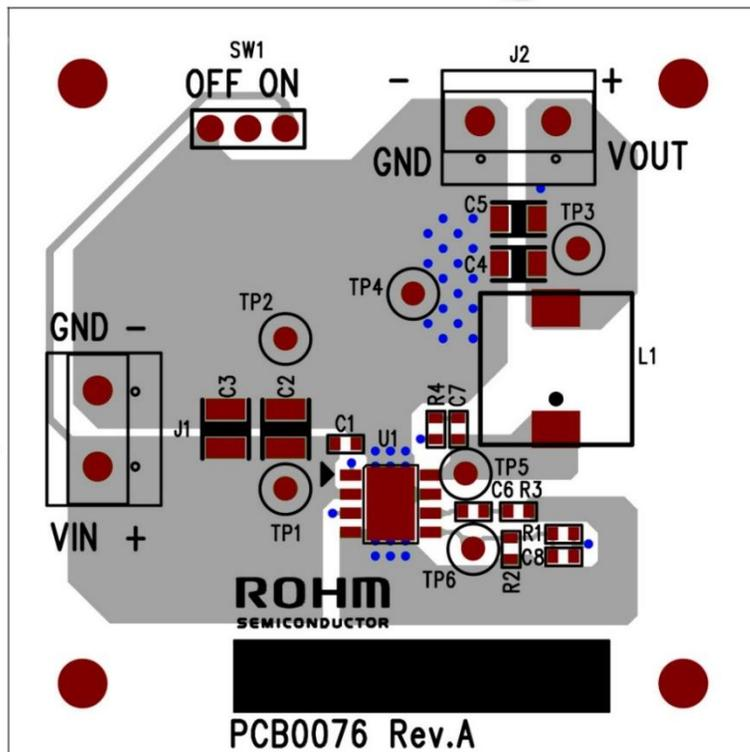
Figure 6. Top Silk Screen and Layout (Top view)
