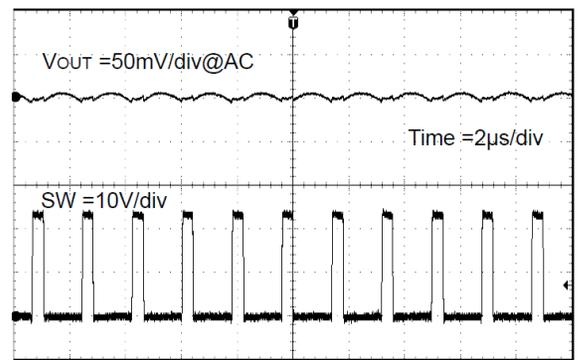
Figure 14. Output Voltage Ripple Wave
