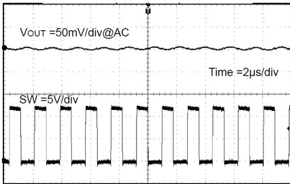
Figure 13. Output Voltage Ripple Wave
