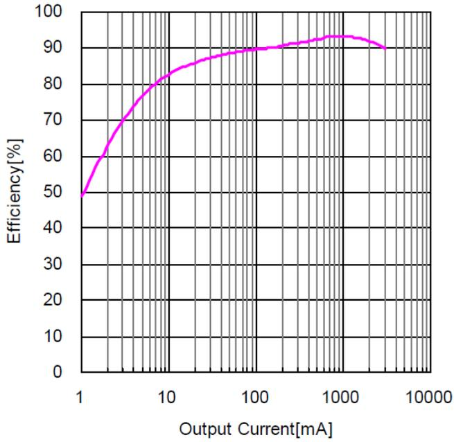
Figure 11. Efficiency vs Load Current
