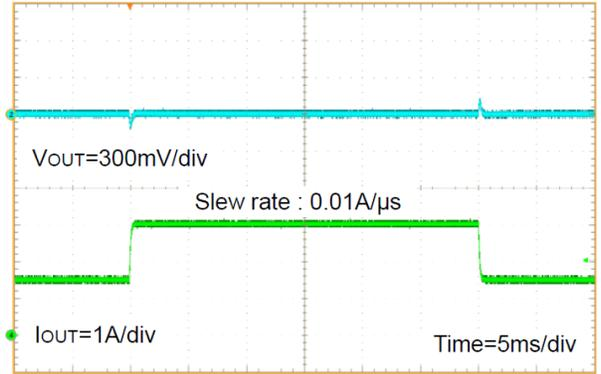
Figure 16. Load Transient Characteristics
