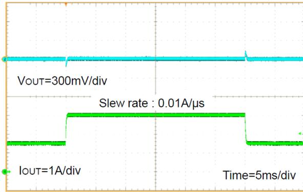
Figure 15. Load Transient Characteristics
