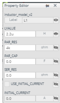
(a) Property editor (b) Equivalent circuit Figure 5. Inductor property editor and equivalent circuit
