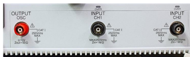
Figure 5. Each terminal electrically insulated from chassis
