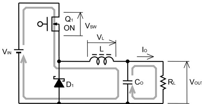
Fig. 1: Basic Buck Converter Circuit Switching Element ON
