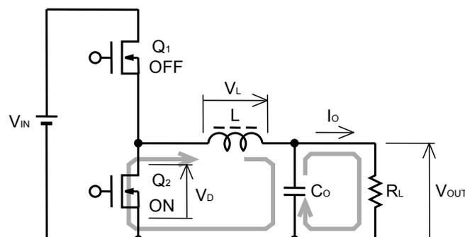
Fig. 4: Basic circuit configuration of a buck converter using synchronous rectification power conversion. In this example, the upper switching element is in OFF-state.
