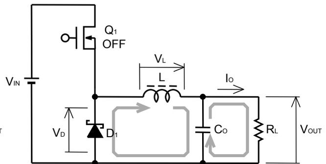
Fig. 2: Basic Buck Converter Circuit Switching Element OFF
