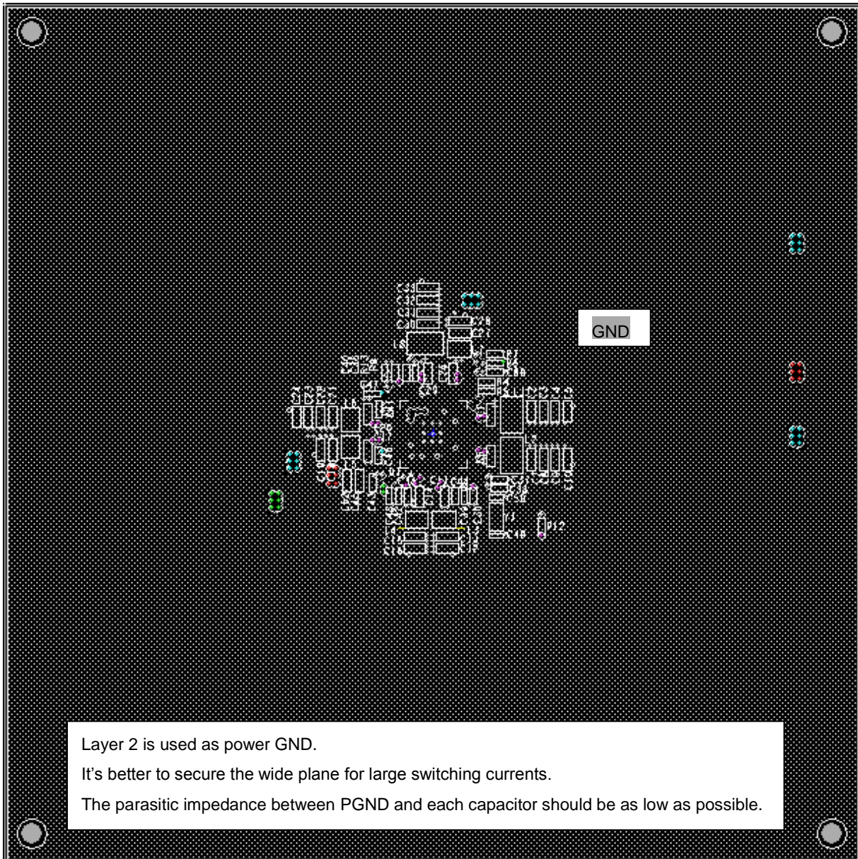
Figure 4.7 BD71837AMWV Reference Board Outline (Layer 2)
