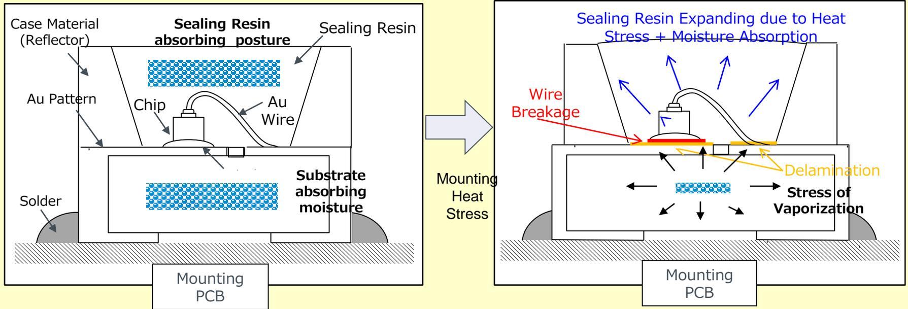
When the product is absorbing the moisture, the vaporized stream (by the heat of reflow) will go out, its stress will lift up the sealing resin from the bottom and result in breakage of wire bonding.
