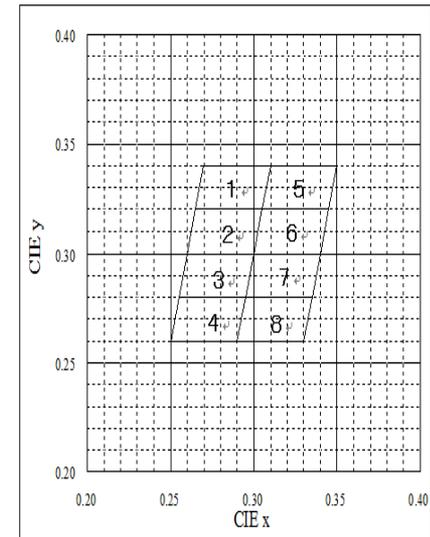
Chromaticity sorting is the value of mixed lighting when applying determined current on products.
