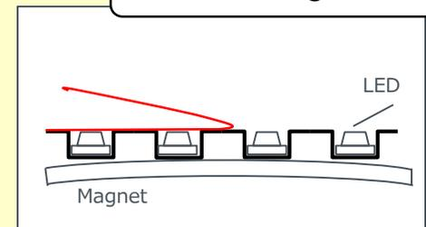
For super small products, it may paste on tape due to static electricity because of the operational environment. In the case, it can solve the problem by installing a magnet on the mounting machine.
