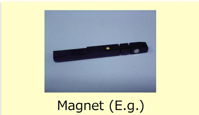
Magnet is used on the mounting machine for picking-up(E.g.)
