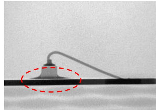
If the peak temperature is too high (excessive), it may cause delamination between Ag paste and circuit board due to warpage of printed wiring circuit board or expansion of resin. And if the temperature gradient of temperature rising/falling is large, it can also cause delamination, so please use it in 1~3°C/sec.
