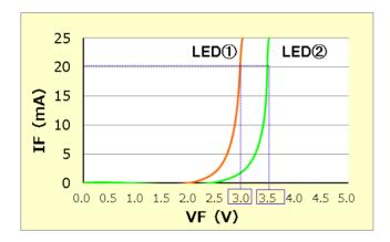
If LEDs with different VF values are driven in a circuit connected in parallel, such as LED ①(VF=3.0V/IF=20mA) and LED ② (VF=3.5V/IF=20mA), the current flowing to the LED with low VF values will be concentrated and cause differences in luminous intensity.
