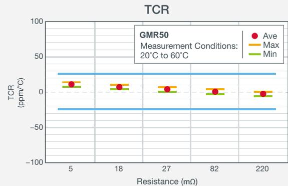
Achieves superior TCR characteristics even in the low resistance region by adopting a high performance alloy for the metallic resistive element
