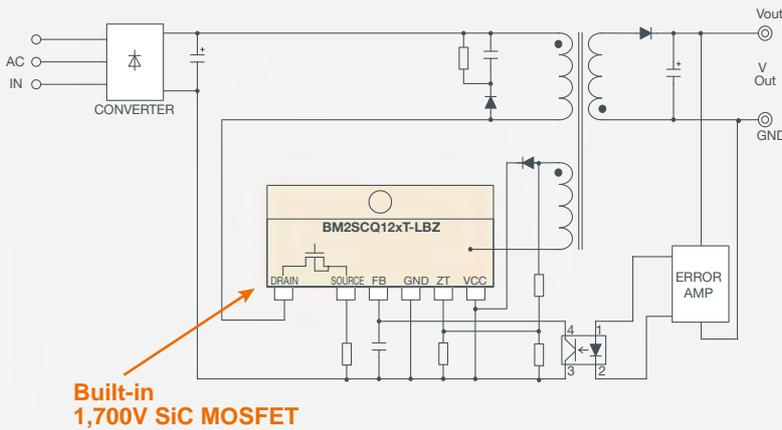
AC/DC converter integrates a 1,700V SiC MOSFET and SiC-dedicated controller
