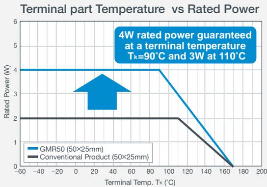
The GMR50 delivers the industry's highest rated power of 4W at a terminal temp.  $T_k=90^\circ\text{C}$  and even 3W at  $T_k=110^\circ\text{C}$  in the compact 5.0×2.5mm size
