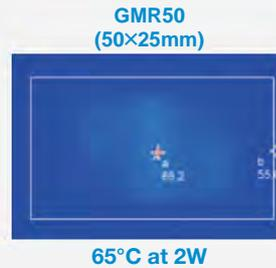
Optimized electrode structure and resistive element design significantly reduce heat generation
