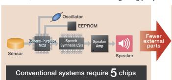
LAPIS Technology MCUs with speech output function incorporate an oscillator, EEPROM, speech synthesis LSI, speaker amp, and other peripheral components, contributing to set miniaturization.
