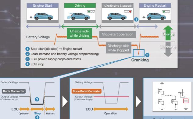
The buck converter stops the ECU during battery voltage cranking
