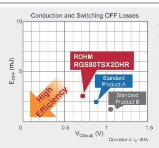
The RGS series was developed with an emphasis on low conduction loss. This enables greater power savings in applications such as PTC heaters and electric compressors.
