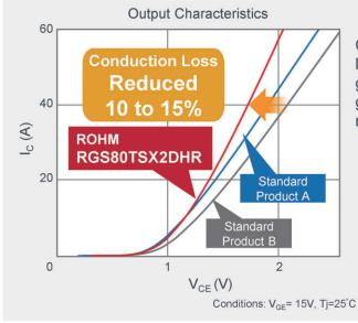
Class-leading\* low conduction loss suppresses heat generation and contributes to greater application miniaturization.
