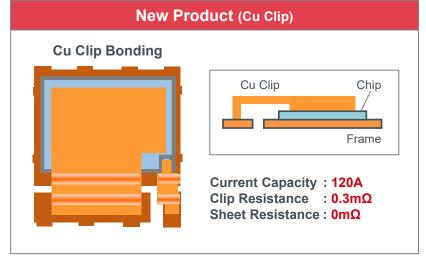
Adopting a Cu clip structure improves specifications for current capacity and package resistance
