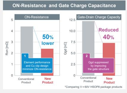
Simultaneously improves gate charge capacitance, which has a trade-off relationship with ON-resistance
