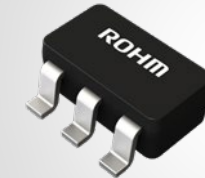
BD7xxL05G-C series SSOP5 Package (2.9 × 2.8 × 1.25mm)
