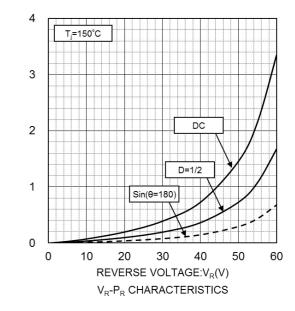
REVERSE POWER DISSIPATION:P<sub>R</sub>(W)
