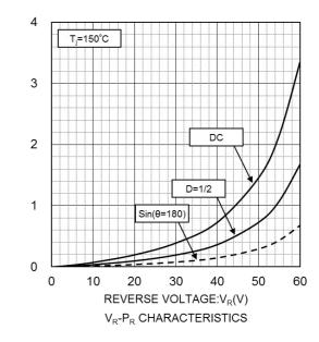
REVERSE POWER DISSIPATION:P<sub>R</sub>(W)
