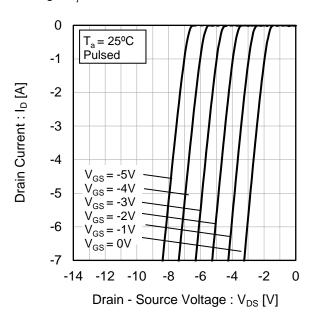
Fig.9  $T_i = 25^{\circ}C$  3rd Quadrant Characteristics
