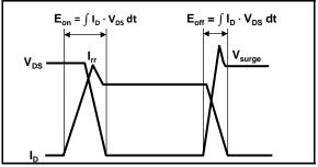
Fig.2-2 Waveforms for Switching Time
