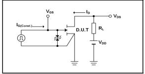
Fig.2-1 Switching Characteristics Measurement Circuit
