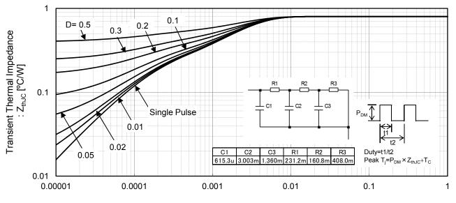
Fig.16 Transient Thermal Impedance
