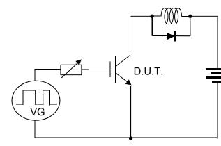
Fig.17 Inductive Load Switching Circuit
