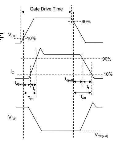
Fig.18 Inductive Load Switching Waveform
