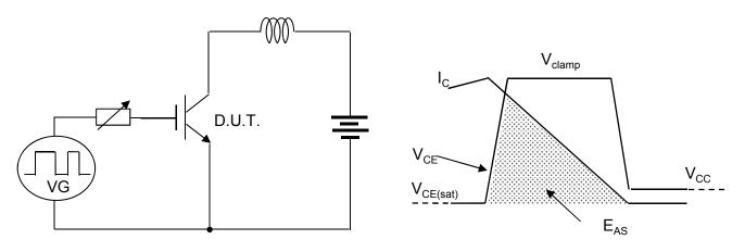
Fig.19 Self Clamped Inductive Switching Ciruit
