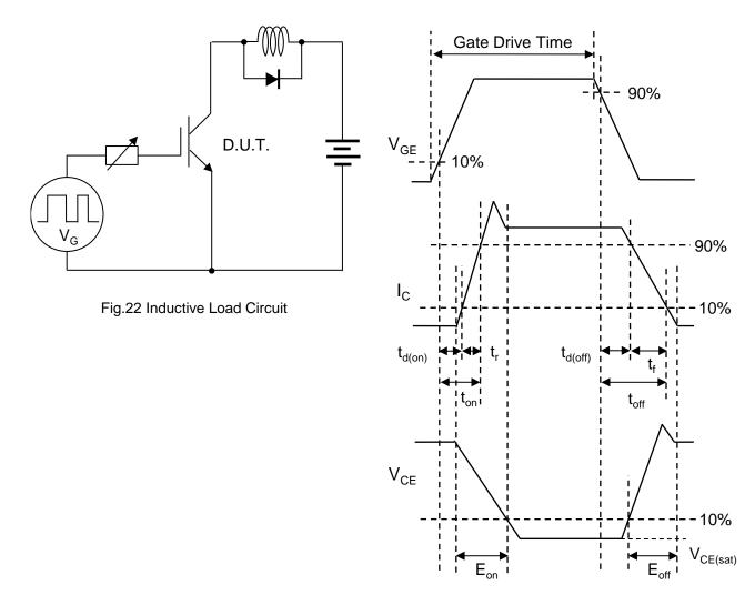
Fig.23 Inductive Load Waveform
