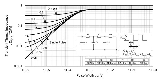
Fig.21 Typical IGBT Transient Thermal Impedance
