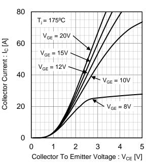
Fig.6 Typical Output Characteristics
