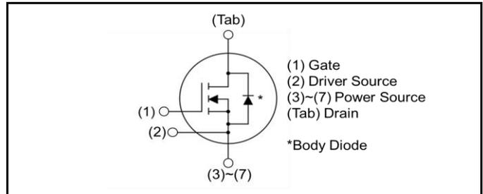
Please note Driver Source and Power Source are not exchangeable. Their exchange might lead to malfunction.
