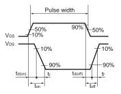
Fig.1-2 Switching waveforms
