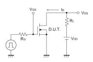
Fig.1-1 Switching time measurement circuit
