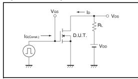
Fig.3-1 Avalanche Measurement Circuit
