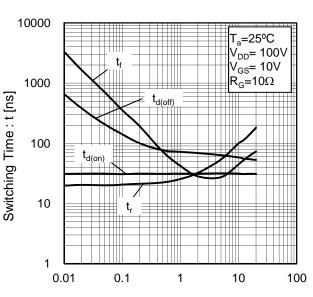
Fig.18 Switching Characteristics
