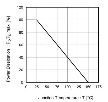
Fig.1 Power Dissipation Derating Curve
