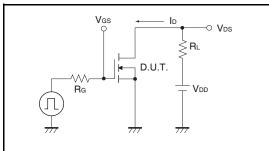
Fig.2-1 Gate Charge Measurement Circuit
