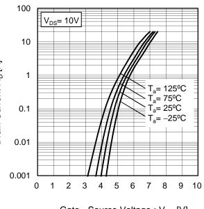
Fig.9 Typical Transfer Characteristics
