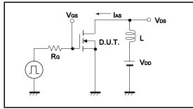
Fig.4-1 dv/dt Measurement Circuit
