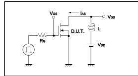
Fig.5-1 di/dt Measurement Circuit
