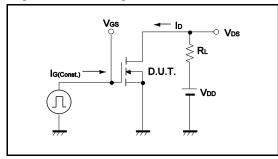
Fig.3-1 Avalanche Measurement Circuit
