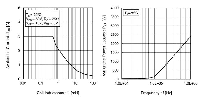
Fig.4 Avalanche Current vs Inductive Load
