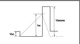
Fig.5-2 di/dt Waveform
