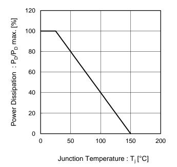
Fig.1 Power Dissipation Derating Curve
