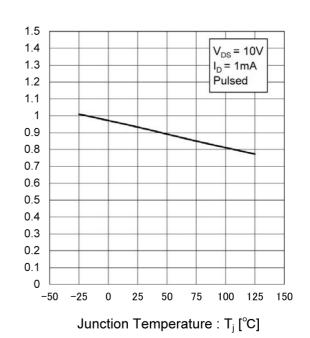
Gate Threshold Voltage: V<sub>GS(th)</sub> [V]
