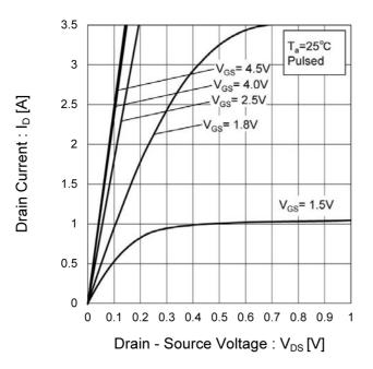
Fig.6 Typical Output Characteristics(II)
