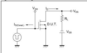
Fig.6-1 Avalanche Measurement Circuit
