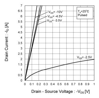
Fig.6 Typical Output Characteristics(II)
