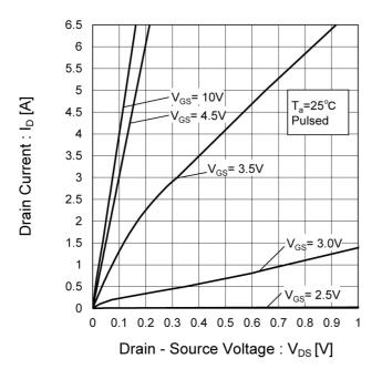
Fig.6 Typical Output Characteristics(II)
