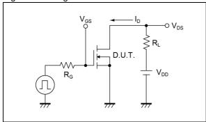
Fig.2-1 Gate Charge Measurement Circuit
