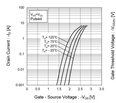
Fig.9 Gate Threshold Voltage vs.
