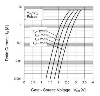
Fig.9 Gate Threshold Voltage vs.
