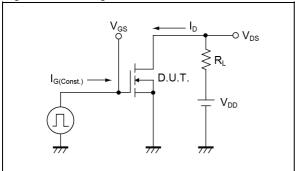
Fig.3-1 Avalanche Measurement Circuit
