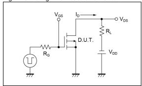
Fig.5-1 Gate Charge Measurement Circuit
