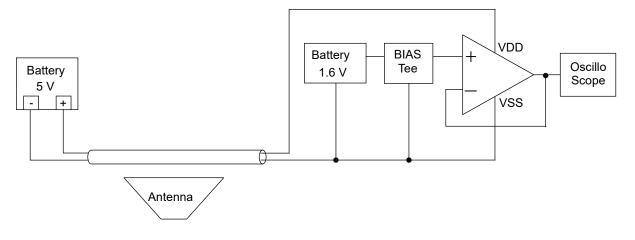
Figure 26. Measurement Circuit of EMI Evaluation
