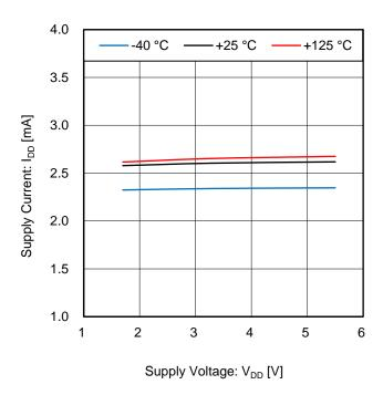
Figure 1. Supply Current vs Supply Voltage
