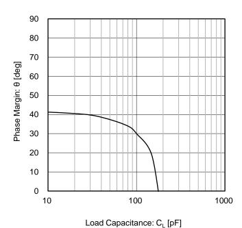
Figure 23. Phase Margin vs Load Capacitance ( $V_{DD} = 5 \text{ V}, \text{ G} = 40 \text{ dB}$ )
