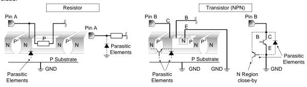
Figure 31. Example of Monolithic IC Structure
