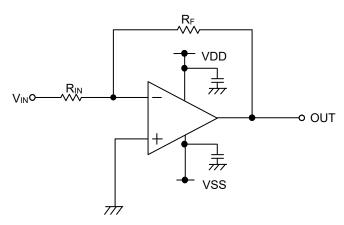
Figure 29. Inverting Amplifier Circuit
