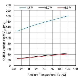
Figure 4. Output Voltage High vs Ambient Temperature (VoH = VDD - VOUT, IOUT = 1 mA)
