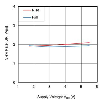
Figure 19. Slew Rate vs Supply Voltage (Ta =  $25 \, ^{\circ}\text{C}$ )
