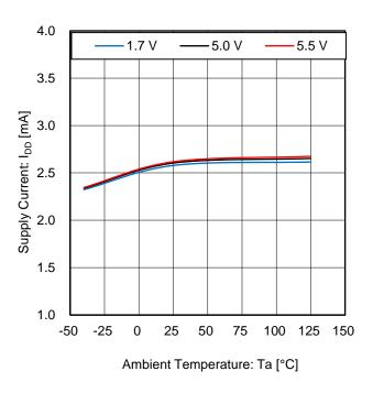
Figure 2. Supply Current vs Ambient Temperature
