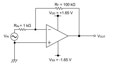
$$V_{OUT} = -\frac{R_F}{R_{IN}} V_{IN}$$
