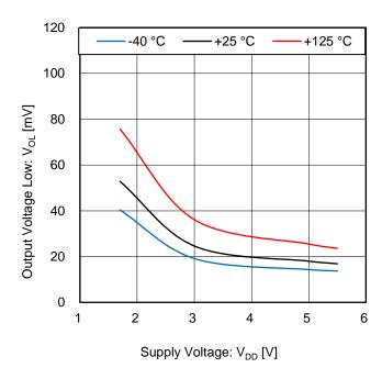
Figure 5. Output Voltage Low vs Supply Voltage (Iout = 1 mA)
