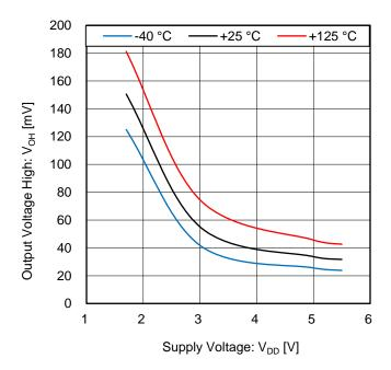
Figure 3. Output Voltage High vs Supply Voltage (VoH = VDD - VOUT, IOUT = 1 mA)
