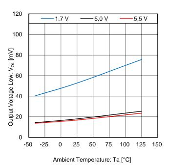
Figure 6. Output Voltage Low vs Ambient Temperature (Iout = 1 mA)
