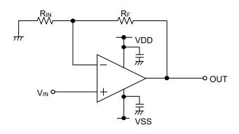
Figure 30. Non-inverting Amplifier Circuit
