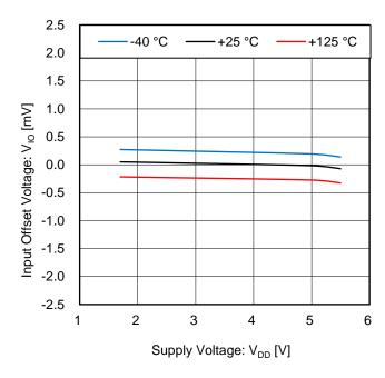
Figure 11. Input Offset Voltage vs Supply Voltage  $(V_{ICM} = V_{DD}/2, E_K = -V_{DD}/2)$
