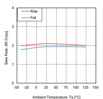
Figure 20. Slew Rate vs Ambient Temperature (V<sub>DD</sub> = 5 V)
